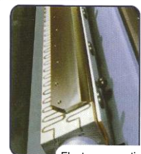
Electro magnetic clamping (EL)
